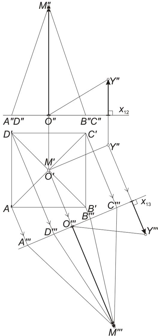
To obtain the view of the pyramid in the given direction, using projection plane transformation, we need to introduce a projection plane perpendicular to  $OY$ . The projecting lines in this view are parallel to  $OY$ , and thus, to get the required view, our task is to transform  $OY$  into a projecting line.
