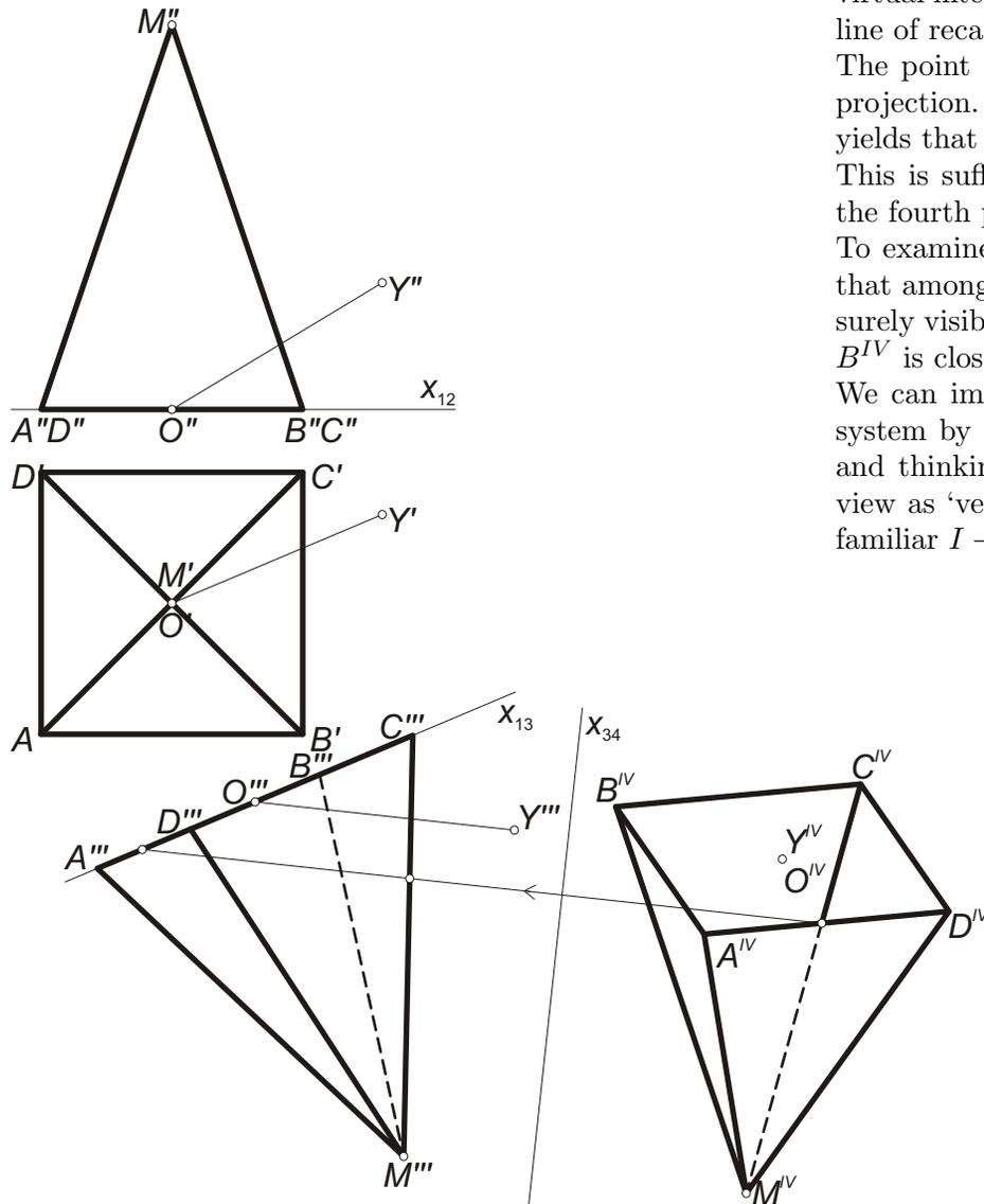
To examine the visibility in the fourth view, we examine the virtual intersection point of the edges  $AD$  and  $MC$ . Drawing its line of recall, we obtain the third projections of the two points. The point farther from  $x_{34}$  covers the other one in the fourth projection. In our case it holds for the point on  $AD$ , which yields that near this virtual intersection point,  $AD$  covers  $MC$ . This is sufficient to determine the visibility of the pyramid in the fourth projection.
