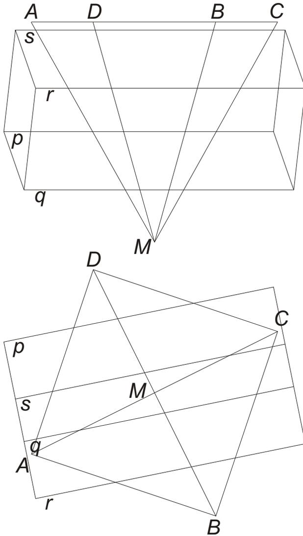
We transform the prism in a way that its sidelines  $p, q, r$  and  $s$  become projecting lines:
