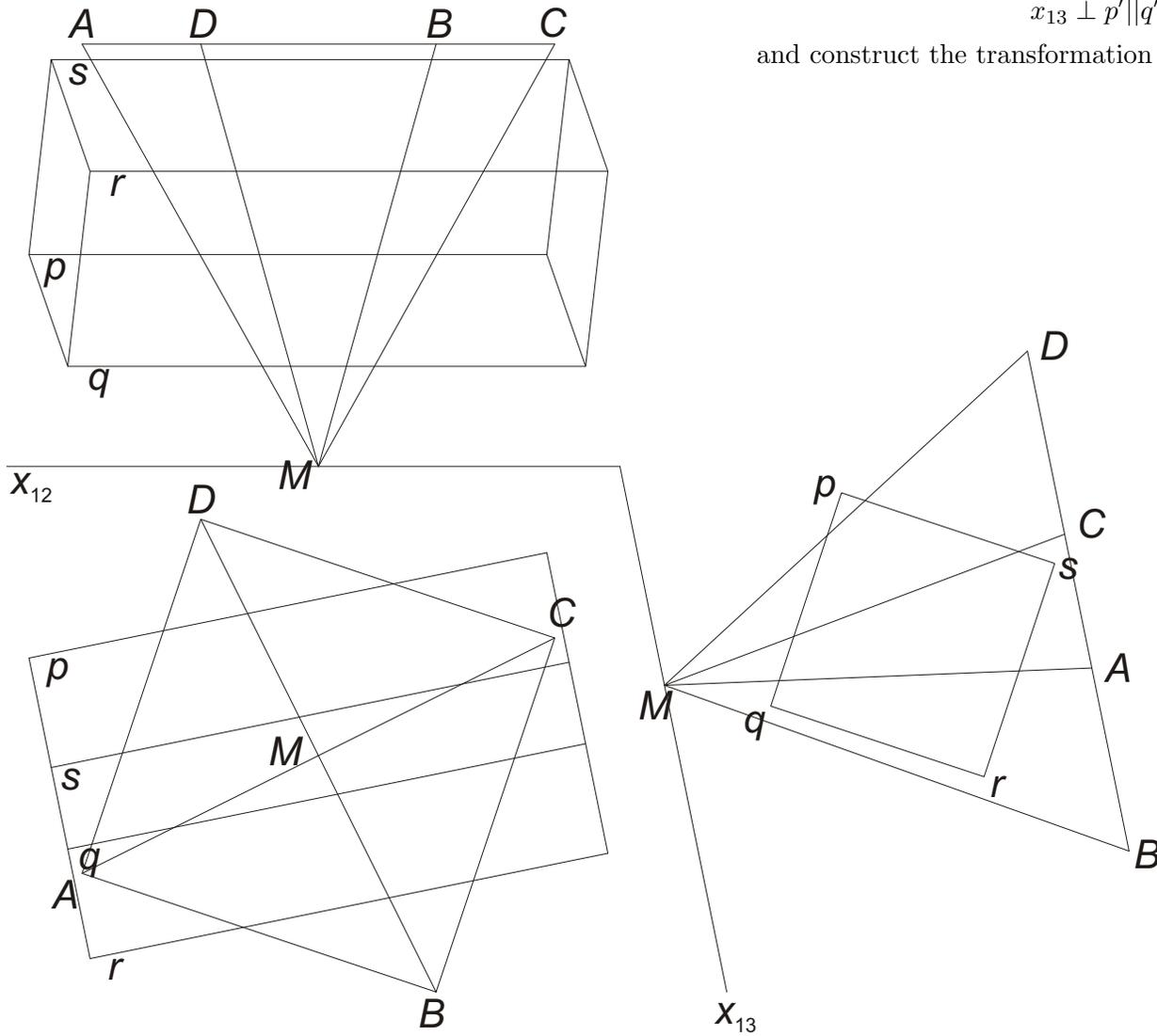
We construct the intersection points of the edges of the pyramid and the prism. These can be found in the third projection, and then, using their lines of recall, their horizontal and vertical projections can be constructed as well. Finally, we make a table showing the incidence properties of the points: on which faces of the polyhedra they lie.
