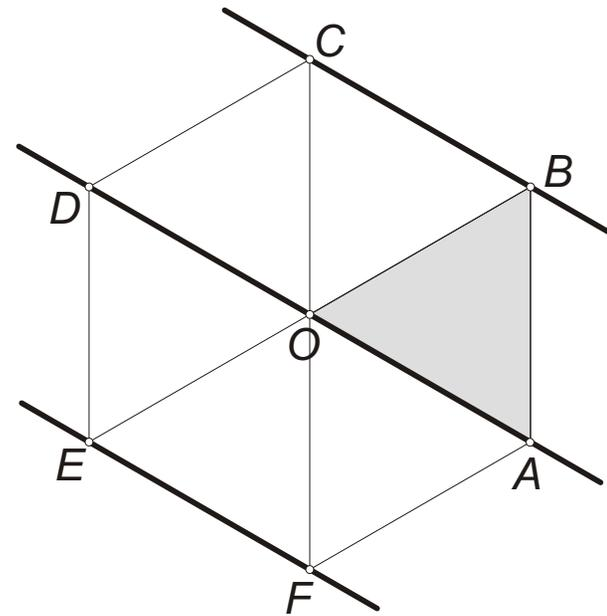
Thus, reflecting  $AB$  about  $O$  we obtain the projections of  $D$  and  $E$ . Then, drawing the lines, through  $B$  and  $E$ , respectively, parallel to the diagonal  $AD$  we obtain the sidelines containing  $BC$  and  $EF$ . Similarly, the lines through  $D$  and  $A$ , respectively, parallel to  $BE$ , contain the edges  $CD$  and  $FA$ .
