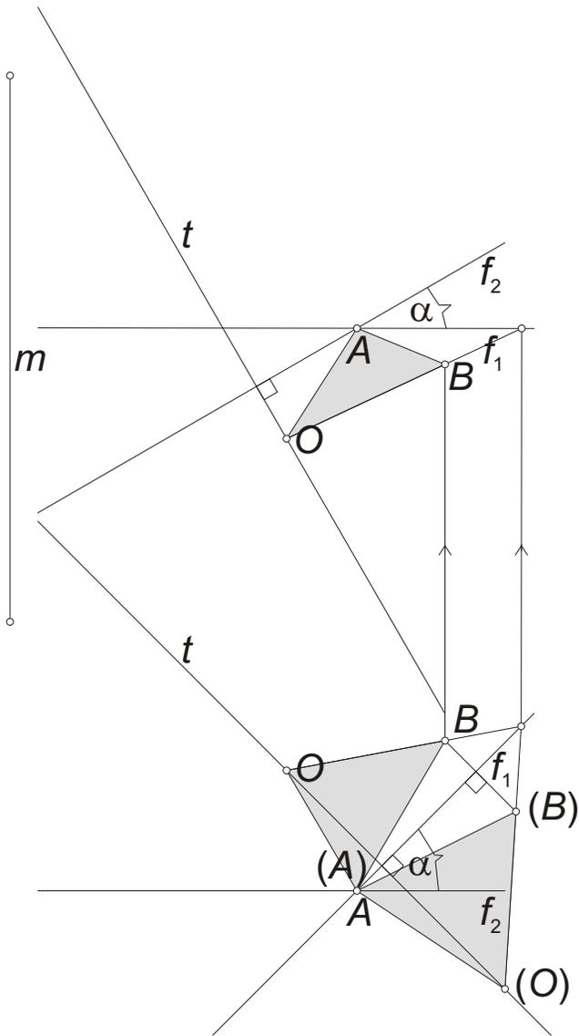
We rotate back the base of the plane, and determine the horizontal and the vertical projections of the triangle  $ABO$ .
