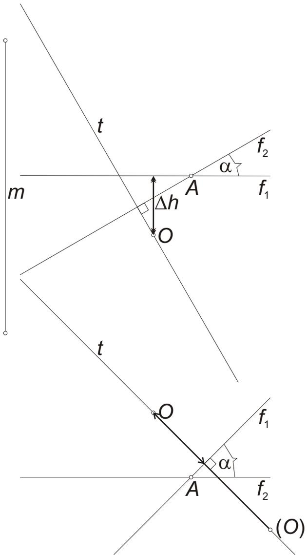
We rotate the plane  $\alpha$ , about  $f_1$  as its axis, into horizontal position.
