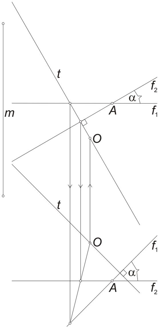
We construct the intersection point  $O$  of the axis  $t$  and the plane  $\alpha$ .
