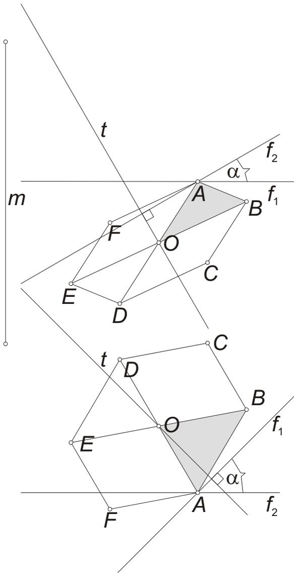
We construct the remaining vertices of the hexagon. We use the fact that in a regular hexagon, the opposite sides are parallel to the diagonal connecting the remaining two vertices and their length is half the length of this diagonal. These properties are preserved by a projection.
