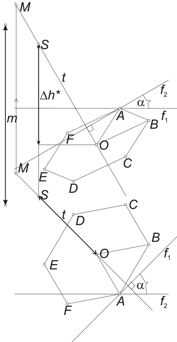
Now we measure the height  $m$  of the pyramid on the axis  $t$  from  $O$ .
