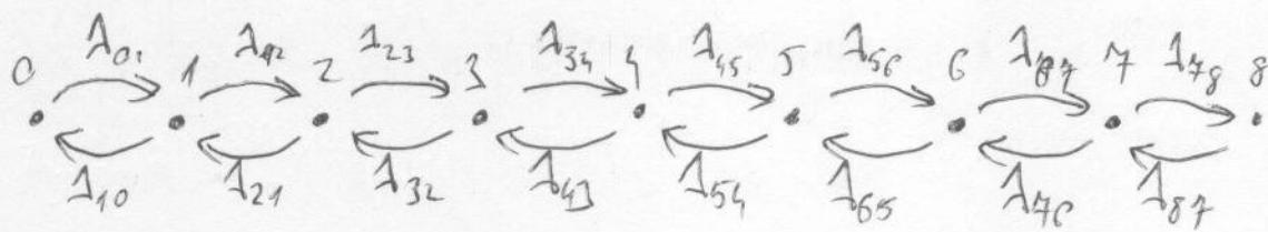
$$\underline{A} = \begin{pmatrix} * & \lambda_{01} & 0 & 0 & \dots \\ \lambda_{10} & * & \lambda_{12} & 0 & \dots \\ 0 & \lambda_{21} & * & \lambda_{22} & \dots \\ 0 & 0 & \lambda_{32} & * & \lambda_{33} \\ \vdots & & & \vdots & \ddots \end{pmatrix}$$
