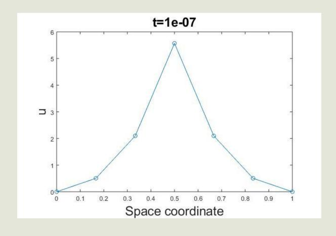
On a finer mesh we obtain the approximation seen in the figure.  $\Delta x = 1/26$ ,  $\Delta t = 10^{-12}$  (10<sup>5</sup>th time step) (stability!)
