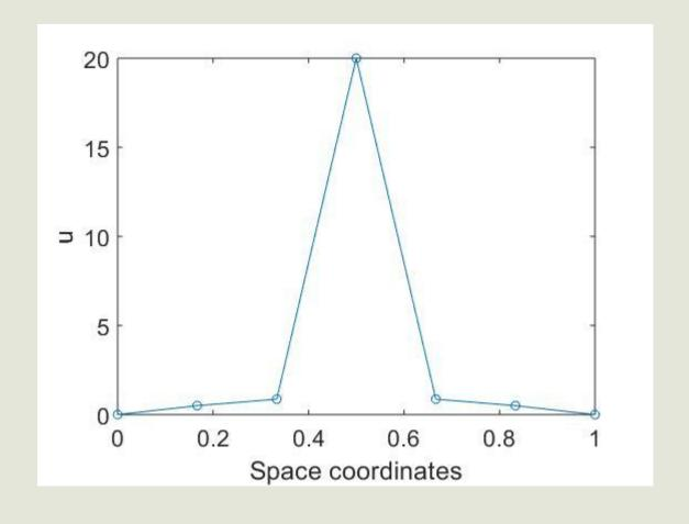
Approximation of the solution at  $t = 10^{-7}$  (10th time level) with the time step  $\Delta t = 10^{-8}$ .
