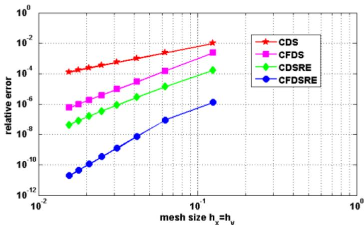
Fig 17: The log-log plot of the errors versus space mesh size for the *Example 2*, obtained by: CDS - red line,  $- \star -$ ; CFDS - magenta line,  $- \blacksquare -$ ; CDSRE - green line,  $- \blacklozenge -$ ; CFDSRE in space - blue line,  $- \bullet -$ .
