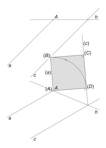
We rotate back the plane and construct the horizontal and the vertical projections of the square base.
