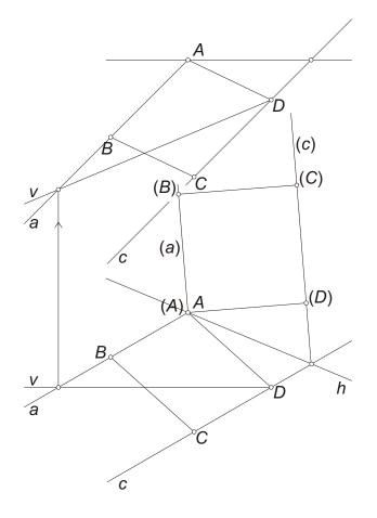
To construct a line perpendicular to a plane we need to know a horizontal and a vertical line of the plane. We already know a horizontal line, h, of the plane of the square, now we choose a vertical line in it. For example, we take the vertical line v, passing through D.
