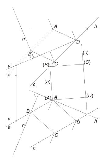
The horizontal/vertical projections of the sidelines containing the lateral edges of the prism are perpendicular to the horizontal/vertical projections of the horizontal/vertical lines of the plane of the base, respectively. For example, n is the line containing BF, and the other lines are parallel to n.
