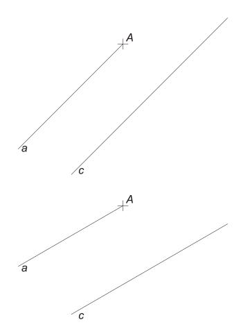
**Exercise.** Given a half line a, starting at A, and a line c parallel to a. Construct a square-based, regular prism ABCDEFGH with base ABCD, if the edge AB lies on a, CD lies on c, and its height is one and the half times the side-length of the base. Show visibility, assuming that the prism is a solid body.
