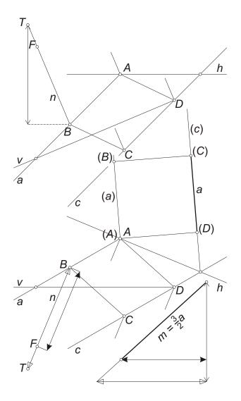
To measure the length of the lateral edges we take an arbitrary auxiliary point T on n, different from B, and construct the difference triangle of the segment BT. The length of the horizontal leg is the distance of B' and T', whereas the length of the vertical one is the difference of the levels of B'' and T''.
