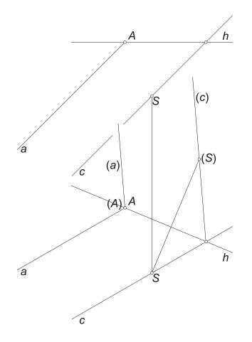
During the rotation, the points of the axis are fixed points, and thus A, and the intersection point of h and a. By connecting the latter one we obtain the rotated copy (c) of c. To construct the rotated copy (a) of the half line a, we draw a half line parallel to (c), starting at A' = (A).
