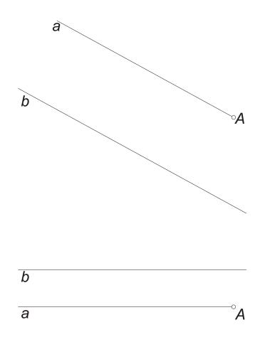
**Exercise.** Given the vertical half line a emanating from A, and the line b, parallel to a. Construct the pentagon-based regular prism  $ABCDEA_xB_xC_xD_xE_x$  if its edge  $AA_x$  lies on a, and  $BB_x$  is contained in b. The height of the prism is equal to the length of the diagonals of the base. From amongst the geometrically feasible solutions, choose the one on the lower level in space. Show visibility assuming that the prism is a solid.
