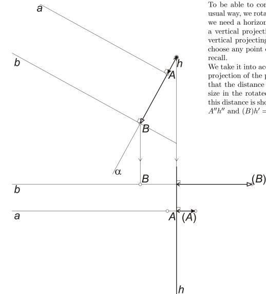
To be able to construct the regular pentagon ABCDE in the usual way, we rotate its plane  $\alpha$  into a horizontal position. First, we need a horizontal line h in  $\alpha$  as the axis of the rotation. In a vertical projecting plane the horizontal lines are exactly the vertical projecting lines of the plane, and thus, as h'', we may choose any point of  $\alpha''$ , and then h' is the corresponding line of recall.
