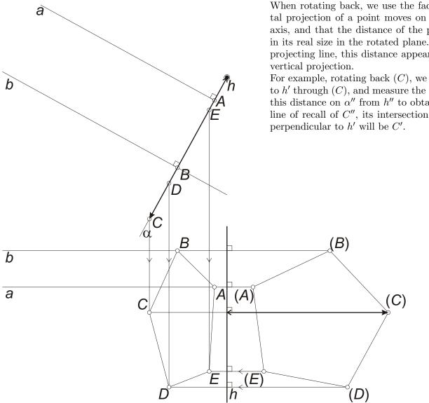
When rotating back, we use the facts, again, that the horizontal projection of a point moves on a line perpendicular to the axis, and that the distance of the point from the axis appears in its real size in the rotated plane. Since the axis is a vertical projecting line, this distance appears in its real size also in the
