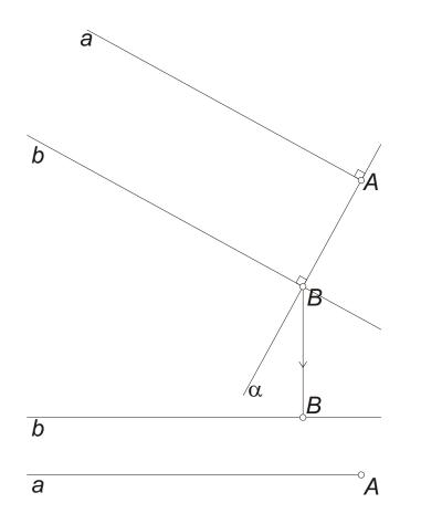
Since the prism is regular, its base ABCDE is perpendicular to the direction of the lateral sides, and thus to a Therefore, as a is a vertical half line, the plane  $\alpha$  of the base is a vertical projecting plane, and  $\alpha'' \perp a''$ .
