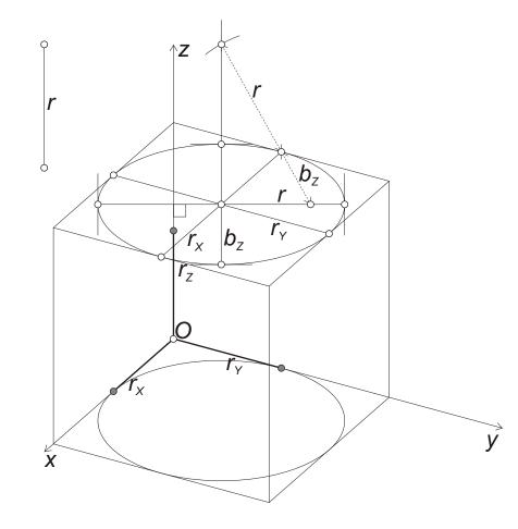
We construct the projections of the incircles of the floor and the roof of the cube. In our case the diameters of the ellipses parallel to the coordinate axes (x and y) are the medians of the faces, and the tangent lines here are the edges of the parallelograms. The major axes of the ellipses are projections of parallel lines of the planes, and thus, they are perpendicular to the z axis; their length is 2r, since in this direction the real lengths are not shortened.
