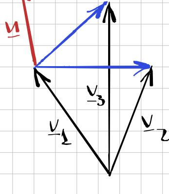
$$\underline{u} = (\underline{v}_2 - \underline{v}_1) \times (\underline{v}_3 - \underline{v}_1)$$
